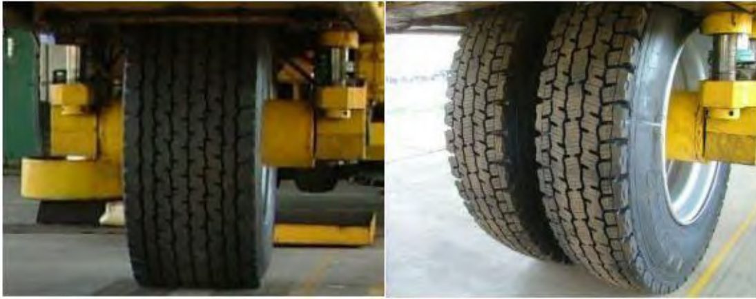
Figure 1: Tire comparison (a) NGWBST and (b) Dual Tire Assembly
